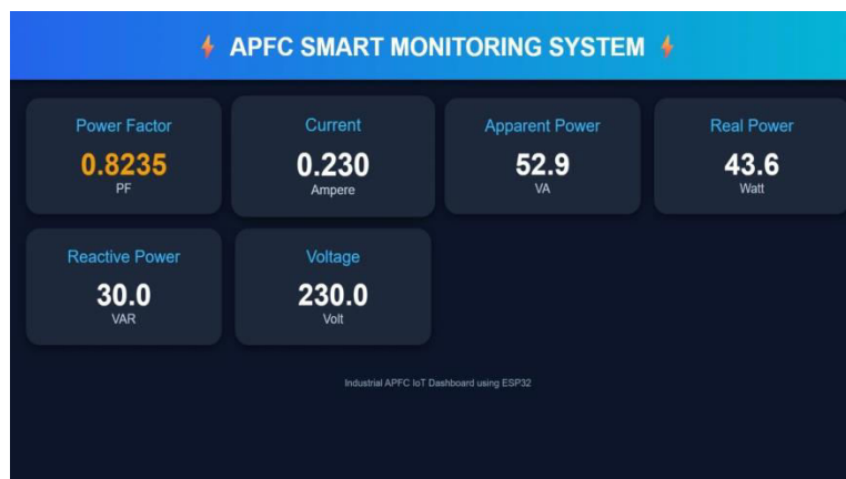
Fig. 4: ESP32 Web Dashboard showing PF = 0.8235 (Amber indicator) - No capacitors connected, natural inductive load condition
